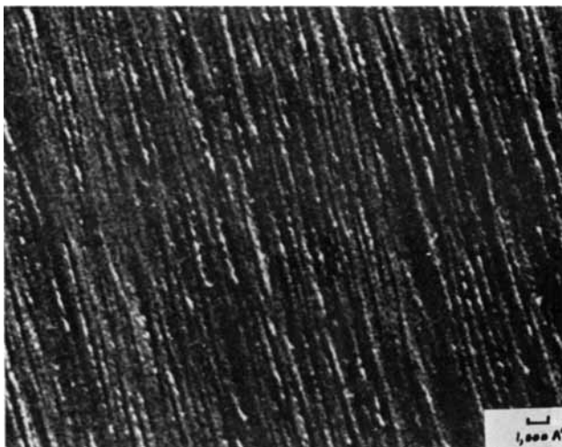
Fig. 17. Detail of fine fibrillar structure in peeled nylon 66. Fibrils are 100–150 Å wide and have a uniform nodular structure of approximately 150 Å.
